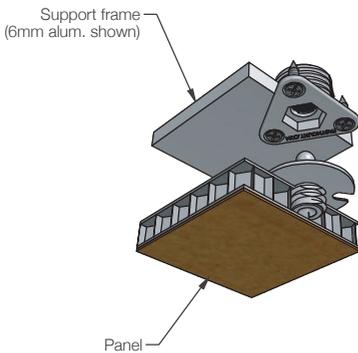
Cutaway exploded view (nts)
